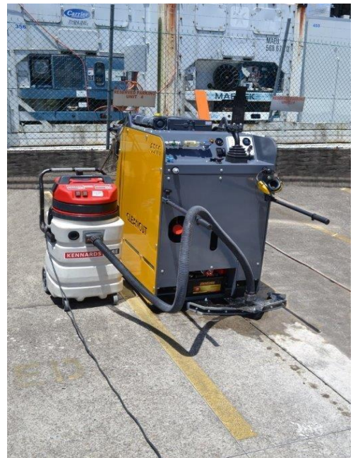
Clean-up using the Cleancut Slurry Clean Up System.
